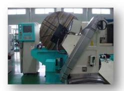
30° Z axis movement design for easy chip disposal (patented)
