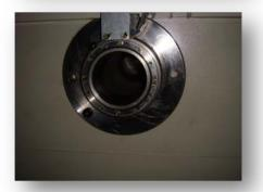
C axis full loop design with 0.001 ° resolution overcome the backlash (patented)
